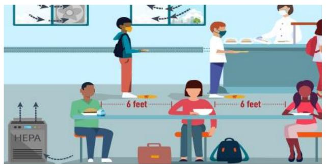
Good ventilation is important, especially in areas where students may not be able to wear masks. Eating meals outside is best. If you need to have students eat in a cafeteria, use methods such as opening windows, maximizing filtration as much as the system will allow and using portable HEPA air cleaners.
